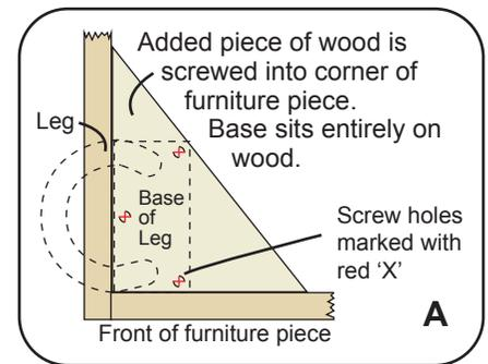
2. **Attaching the Legs:** Turn piece of furniture bottom side up. Position flat top edge of leg against corner of wood as desired. If positioning diagonally, place a mark 2-1/2" from each corner; align corners of base to these marks. Mark screw hole positions. Drill a hole at each position. Use a screwdriver to attach screws.
