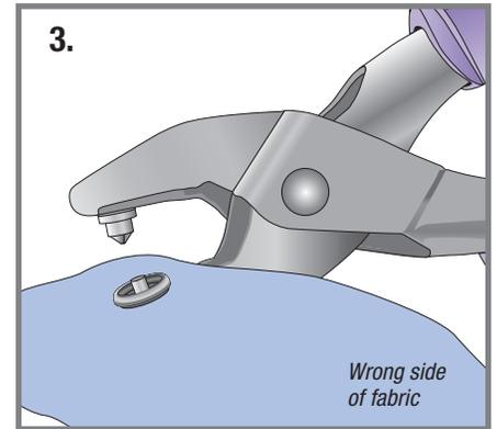
4. Squeeze pliers firmly to apply cap and socket. Check for tightness; squeeze again, if necessary.
