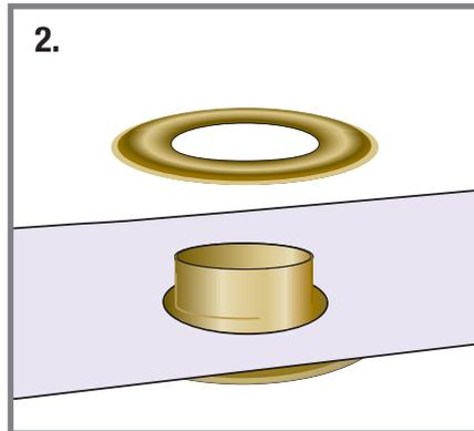
3. With grommet holder at bottom of pliers, place grommet, fabric and washer onto holder.
