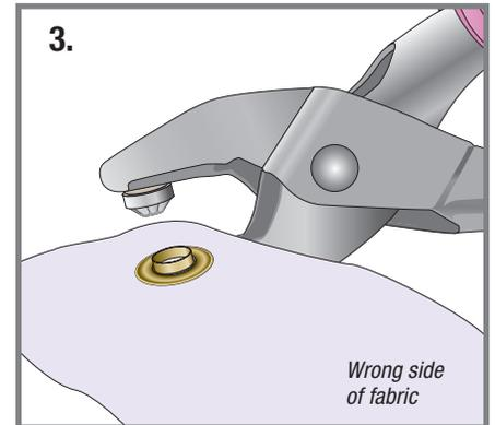
4. Squeeze pliers firmly to apply grommet. Check for tightness; squeeze again, if necessary. The grommet will split and roll back over the washer.
